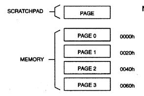
NOTE: Each page is 32 bytes (256 bits). The hex values represent the starting address for each page or register.
