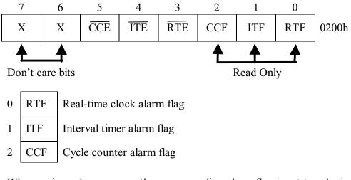
When a given alarm occurs, the corresponding alarm flag is set to a logic 1. The alarm flag(s) is cleared by reading the status register.
